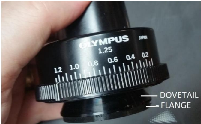
Figure 12 – The BH2-FDR fitted into a BH2-CD condenser
