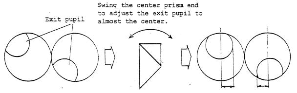
Separate the displacement of left and right exit pupils.
