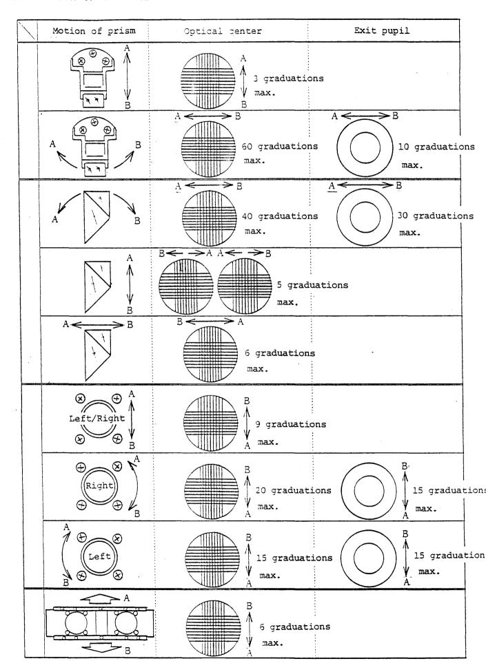
The optical center or exit pupil is displaced in the horizontal direction.
