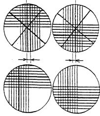
The center prism is excessively or insufficiently moved forward and rearward. Return to 1-2-3 to move the prism appropriately.
