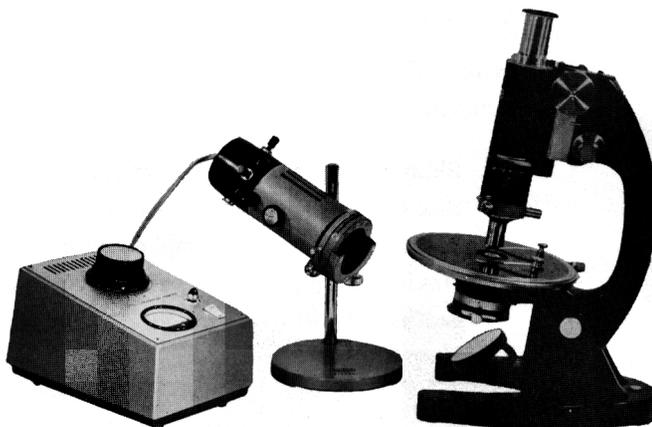
2. Plug-in substage Simple Illuminator Model LSK-4
