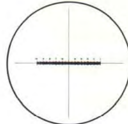
b) Cross 10/100: 10mm in 100 divisions on crosslines
