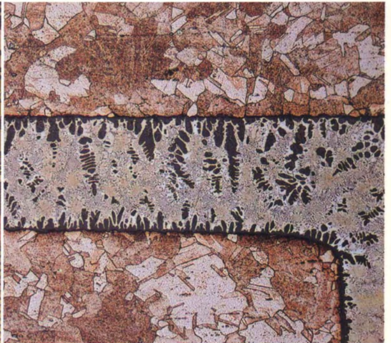
Silver Brazing Filler Metal. Brazing Structure. M SPlan 20x, NFK 2.5x
