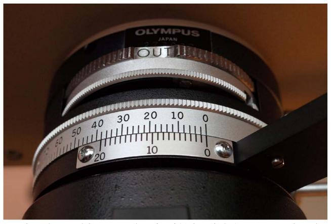
Rotate the analyzer until the vernier scale reads  $\circ.\circ^{\circ}$ . Tighten the locking pin. Insert the analyzer.
