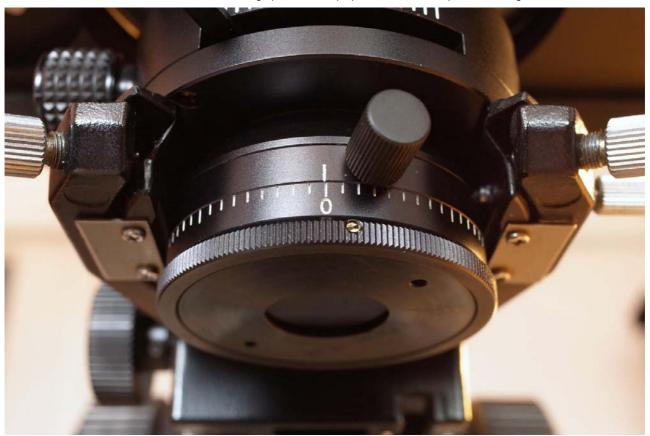
Check that the polarizer's click stop position adjustment screw is locked. Rotate the polarizer until it clicks into o.
