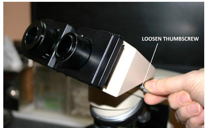
Figure 7 – Loosen mounting thumbscrew (binocular shown)
