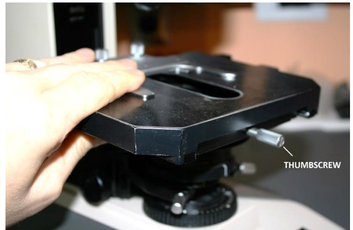
Figure 10 – Remove the stage from stage-mounting ring
