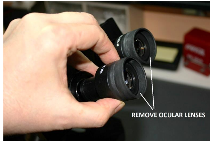
Figure 6 – Remove the ocular lenses from eyepiece tubes
