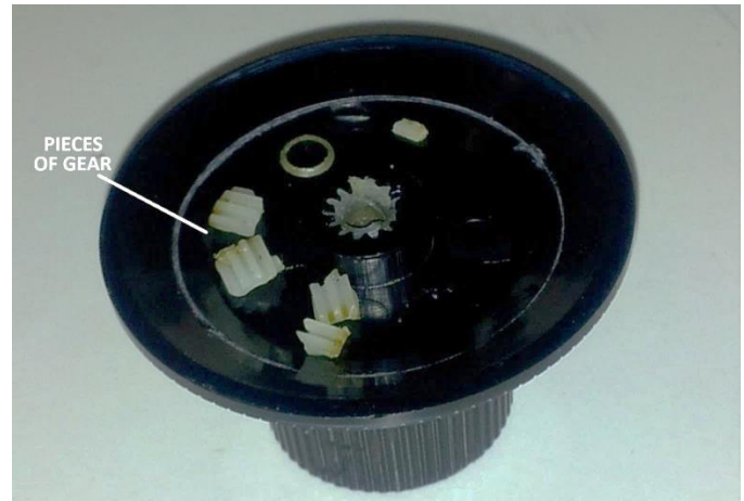
Figure 3 – A fine-focus gear broken during shipping
