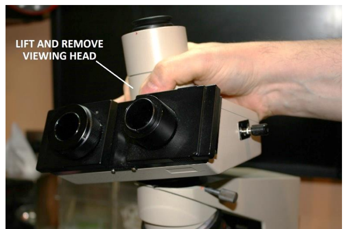
Figure 8 – Remove the viewing head (trinocular shown)
