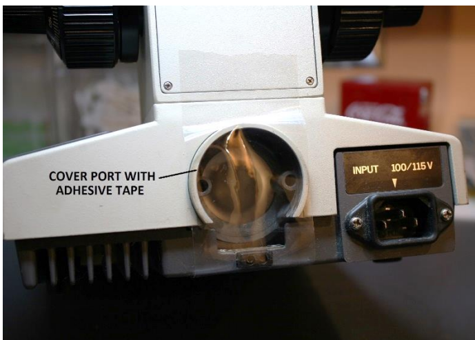
Figure 5 – Cover the exposed lamp-house port
