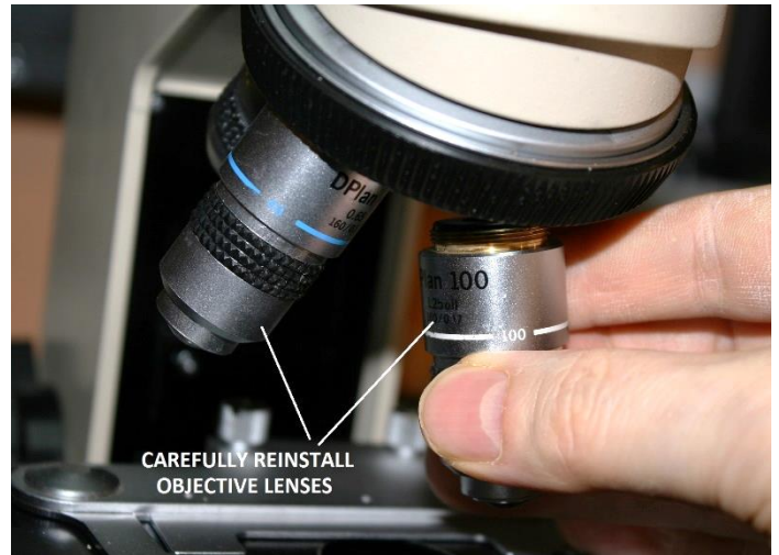
Figure 16 – Reinstall the objective lenses into nosepiece
