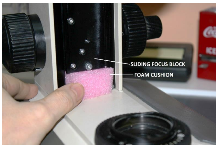
Figure 17 – Place foam below the sliding focus block
