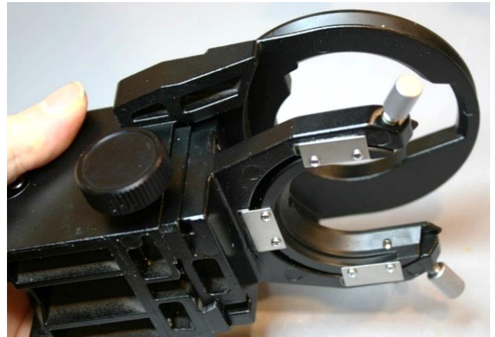
Figure 15 – The substage condenser carrier (w/o condenser)
