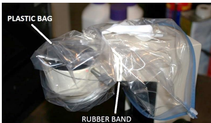
Figure 18 – Protect the top of the arm from dust and debris
