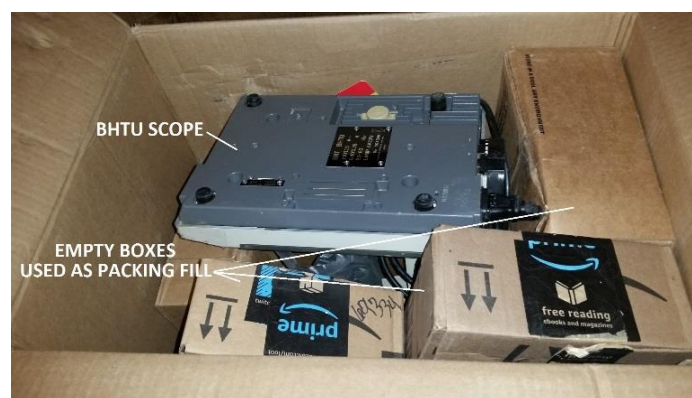
Figure 19 – Very poor packaging of a BHTU stand
