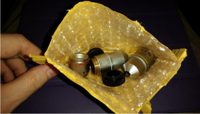
Figure 20 – Incorrect packaging of objectives
