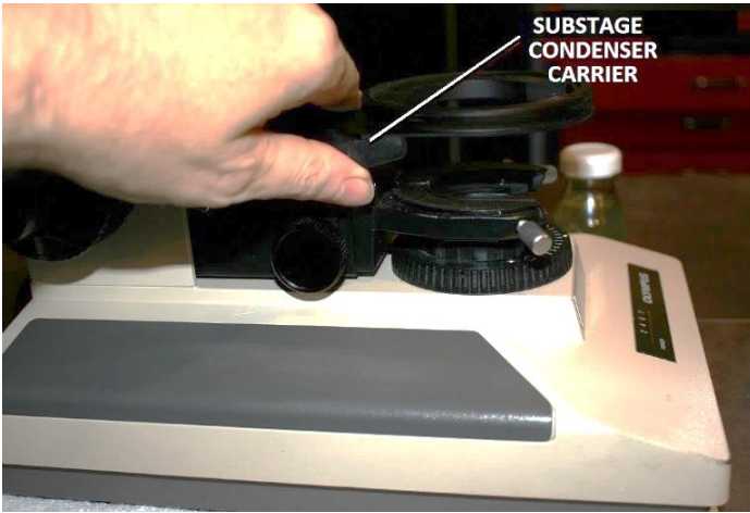
Figure 12 – Lift and remove the substage condenser carrier
