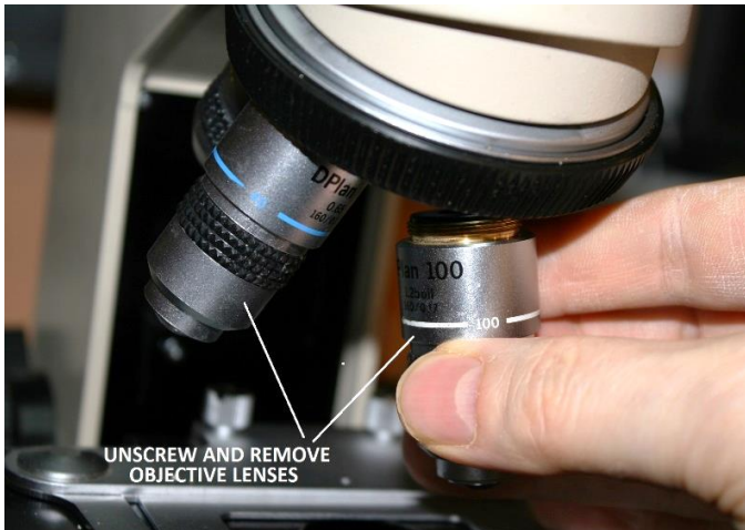
Figure 9 – Remove all objective lenses from the nosepiece
