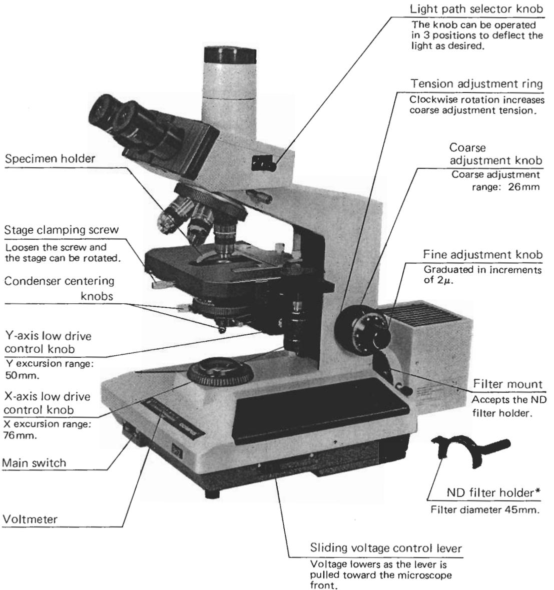
\*Do not disengage the ND filter for about a few minutes after the use, in order to give time to cool. Other filters (e.g. KB-4 provided, etc.) should be inserted into the filter mount at the light exit on the microscope base.
