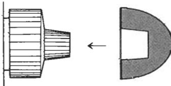
Attaching this cap over the fine adjustment knob increases the sensitivity of the fine focusing motion. (The rubber cap is optionally available.)
