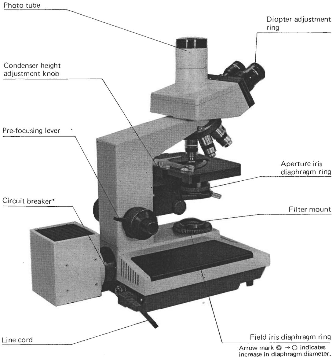
\*This breaker protrudes its central part to cut off the electric power in case of the dimmer circuit trouble (due to short circuit, etc.) or over current. To restore the breaker, press the central part. If the breaker is actuated again, disconnect the line cord from the AC outlet and contact the Olympus Service Center.
